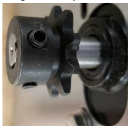
The Motor Sprocket is flush with the Shaft of a Conveyor Motor.
