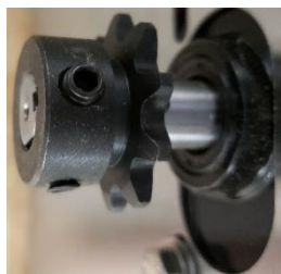
The Front Motor Sprocket is flush with the Shaft Rear Motor Sprocket is aligned with the back end of the Flat.
