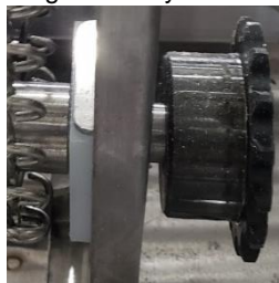
Drive Sprocket is flush with the Shaft of a Standard Conveyor Shaft.
