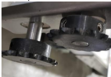
Offset Sprockets: Setscrew on Flat and Round
