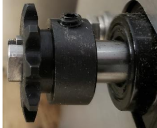
The Front Motor Sprocket is flush with the Shaft Rear Motor Sprocket is aligned with the back end of the Flat.
