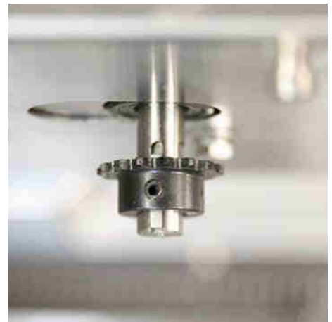
SPLIT-BELT FRONT MOTOR 15 TOOTH, 25 PITCH (2 x ALLEN SET SCREWS)
