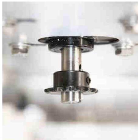
SPLIT-BELT REAR MOTOR 15 TOOTH, 25 PITCH WITH REVERSED ORIENTATION (2 x ALLEN SET SCREWS)
