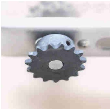
NON SPLIT-BELT CONVEYOR 15 TOOTH, 36 PITCH (2 x ALLEN SET SCREWS)
